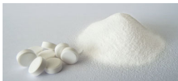
Fig. 1 Pure Vitamin D 3 Powder (100,000 I.U.) and Vitamin D 3 Tablets Composed of PROSOLV® EASYtab Nutra and 5 % of Vitamin D 3 Powder
