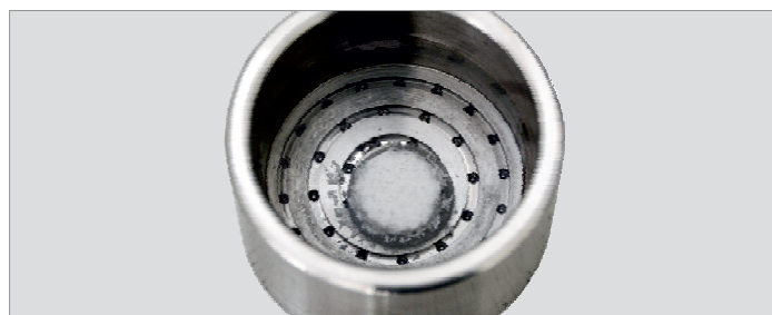
Pic 5 Tablet Containing PVPP after Measurement in Water and Removing of the Upper Glass Filter Disk
