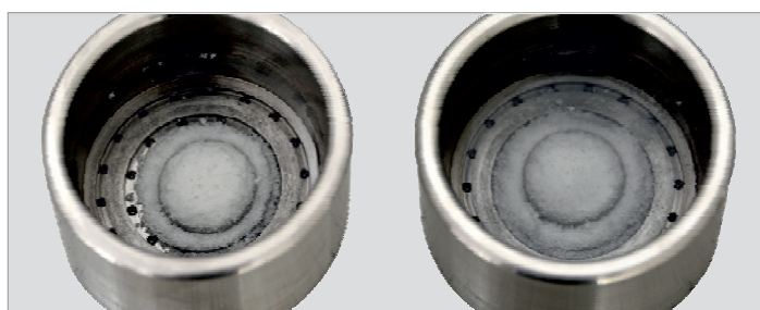
Pic 4 Tablets Containing CCS (left) and SSG (right) after Measurement in Water and Removing of the Upper Glass Filter Disk
