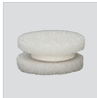
Pic 2 Tablet Between Two Sintered Glass Filter Disks
